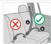
?(?) Can be installed **ONLY** on seats **WITH 3-POINT BELTS!**
